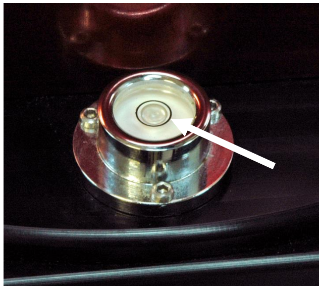
Figure 62: Center the bubble in the black ring for best results.
