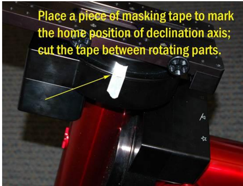
Figure 4: Marking the Paramount’s home position.
