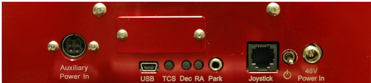
Figure 39: Photograph of the Paramount ME II Electronics Box.
